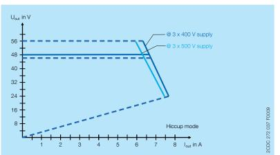
Characteristic curve of output at  $T_a = 25$  °CThe switch mode power supply CP-T 48/5.0 is able to supply at 48 V DC output voltage and
