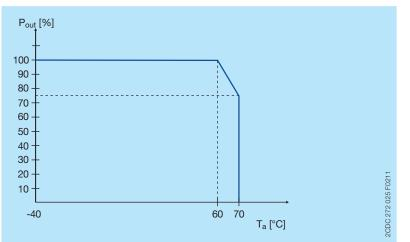
Characteristic curve of temperature at rated load
