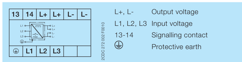
Connection diagram
