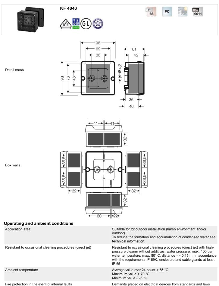
Minimum requirements - Glow wire test in accordance with IEC 60 Page 2 of 3
