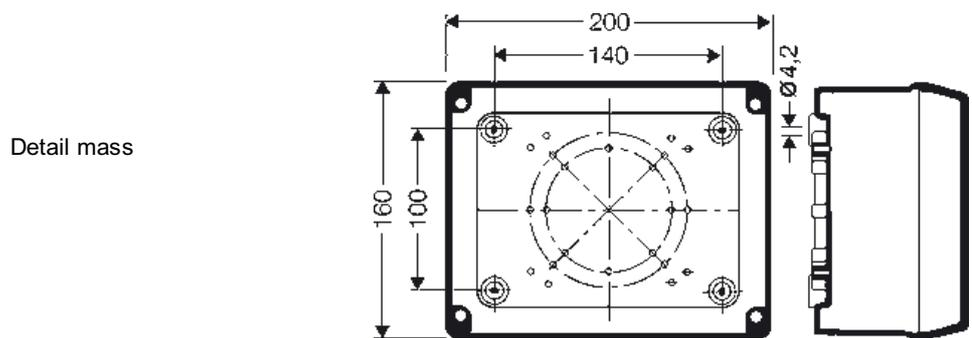
Cable junction box "waterproof" for encapsulating
